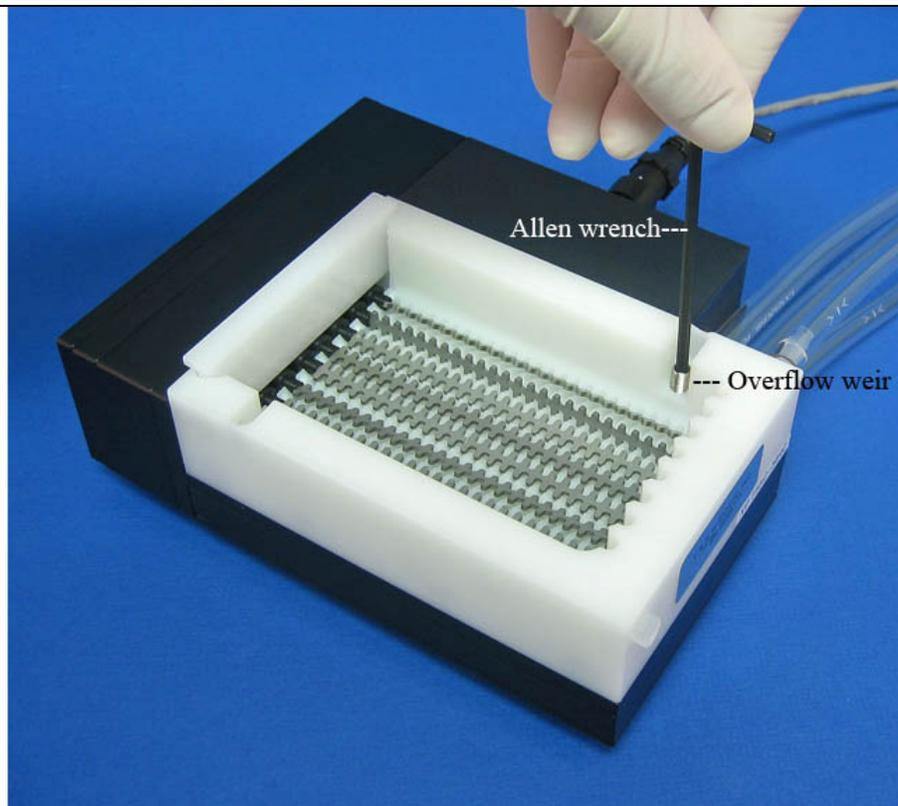
Figure 5. Illustrates the placement of the inlet plug in static operational conditions.
