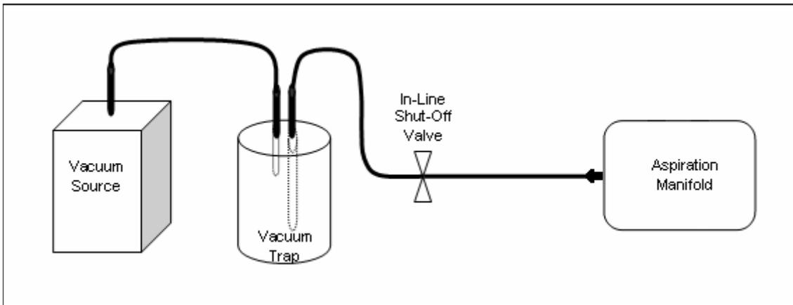
**Figure 2. Connecting the Manifold to Vacuum System.**
